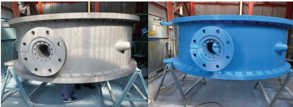
Pictures C: Valve body sandblasted and then painted.
